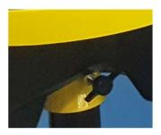
Once the KTP knows its zero pan angle, lock it into position by tightening the knob on the yellow cylinder under the Knight Trainer Pro and by locking the wheels on the stand.
