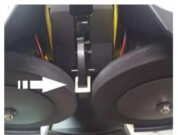
With your Knight Trainer Pro, you received a spacer that sets the ideal gap between the wheels. This spacer slides onto on the finger that passes between the wheels. Be sure to remove the spacer after the wheels have been adjusted.
